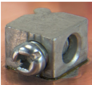
B6A-PCB-45(-RS) SMT mode horizontal screw axis AWG 6-14 65A 75C (0.50" X 0.53" contact surface)
